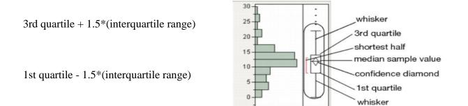
If the data points do not reach the computed ranges, then the whiskers are determined by the upper and lower data point values (not including outliers). The bracket outside of the box identifies the *shortest half*, which is the most dense 50% of the observations (Rousseuw and Leroy 1987).
